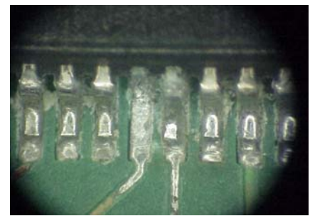
Picture 1: Hand solder flux residues (Not all white residues are corrosive residues.)
