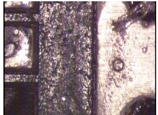
Assembly under pqfn area after steam cleaning: 7.23 \mu\text{g} / \text{in}^2 WOA
